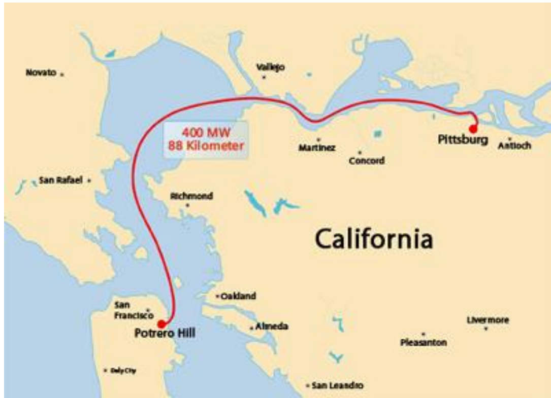
Fig.1. 6 Trans Bay Cable in CA with MMC Technology
