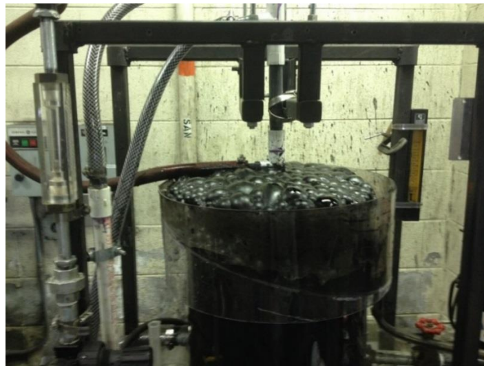
Figure 27. Flotation of a Minus 150 Micron Coal using a Magnetic Sparging System
