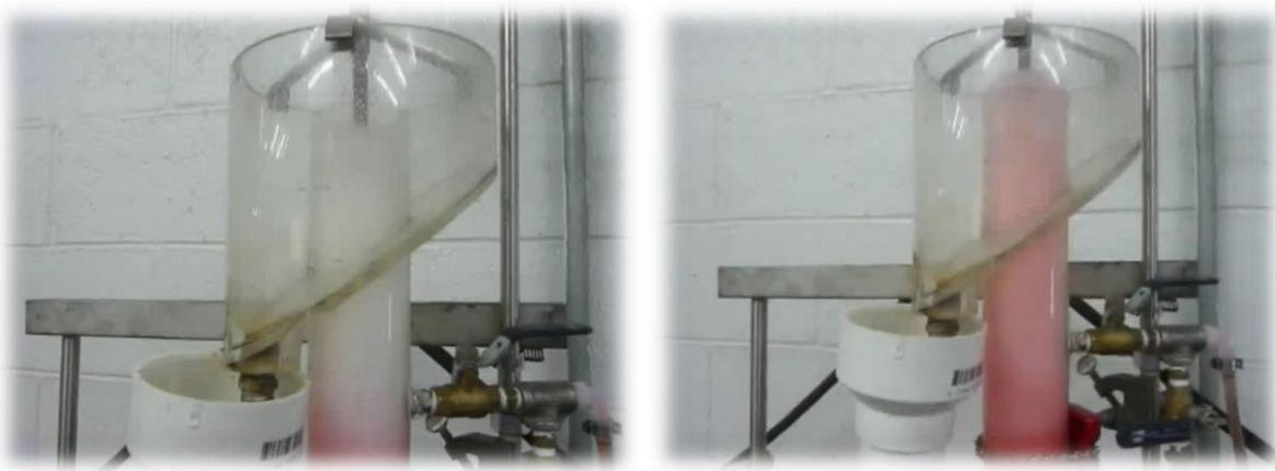
Figure 6. Tracer Study showing the effects of Wash Water Utilization
