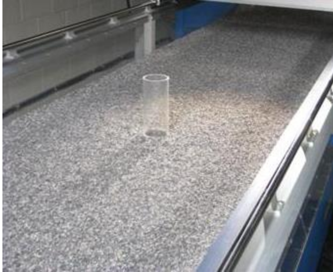
Fig. 2. View of the flume and the model pier.
