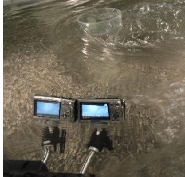
Fig. 3. The cameras recording the scour hole, mounted on the side walls of the flume.
