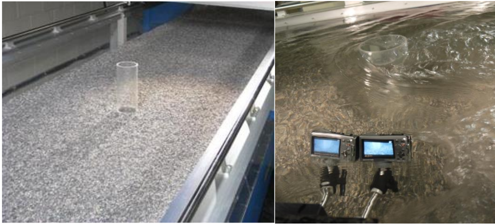
Figure 1. a. View of the hydraulic flume; b. view of the cameras recording the bed during the experiment.
