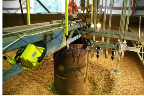
Figure 2. View of the instrumented, 0.61m-wide pier. Flow direction is from right to left. On the centerline upstream of the pier, 4 ADVs and an array of ARFs are visible. Three ARFs on the surface of the pier can be observed.
