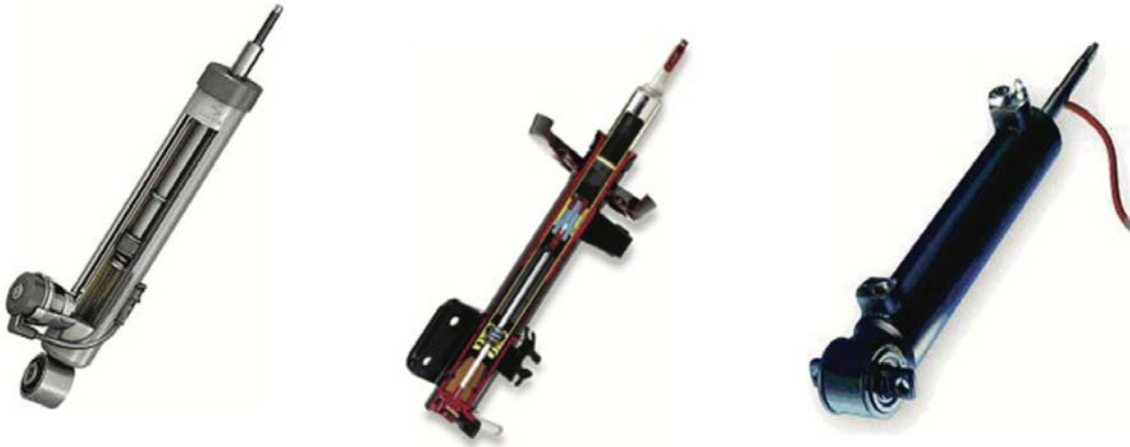
Figure 8: Examples of semi-active damper, (a) Solenoid operated electrohydraulic damper (Sachs). (b) Magnetorheological damper (Delphi). (c) Electrorheological damper (Fluidicon). Used under Fair Use 2016 [4]
