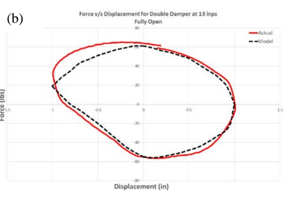
Figure 53: Double damper Force v/s displacement correlation at 13 in/sec for (a) Fully closed valve (b) Fully open valve
