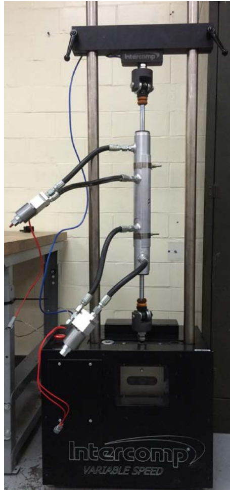
Figure 29: Double damper mounted to Intercomp Dyno
