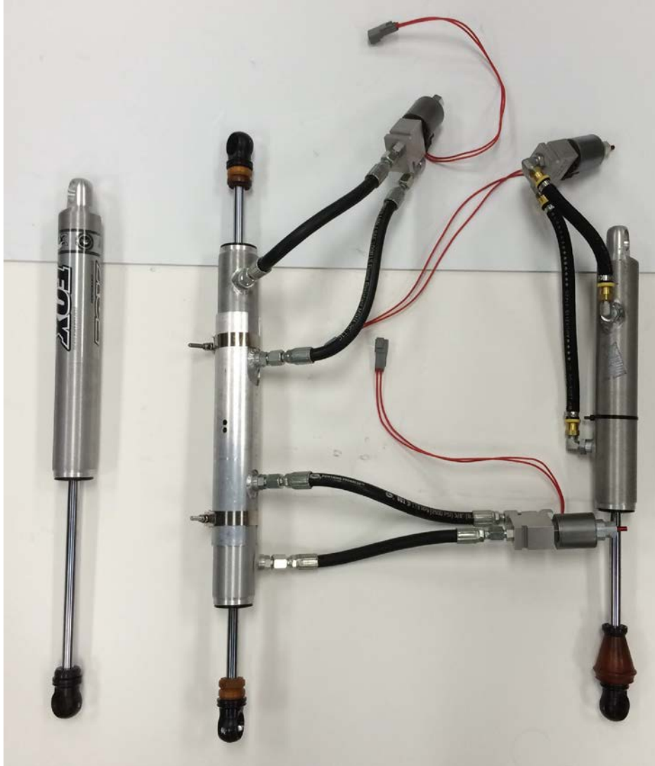
Figure 22: Dampers used from left to right (a) Fox passive damper (b) Double damper (c) Single semi-active damper
