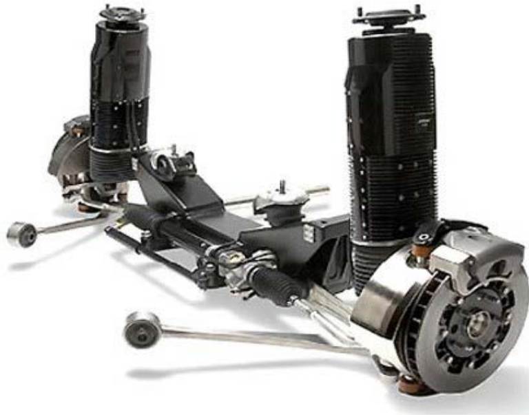
Figure 6: Bose active suspension system. Used under Fair Use 2016 [4]
