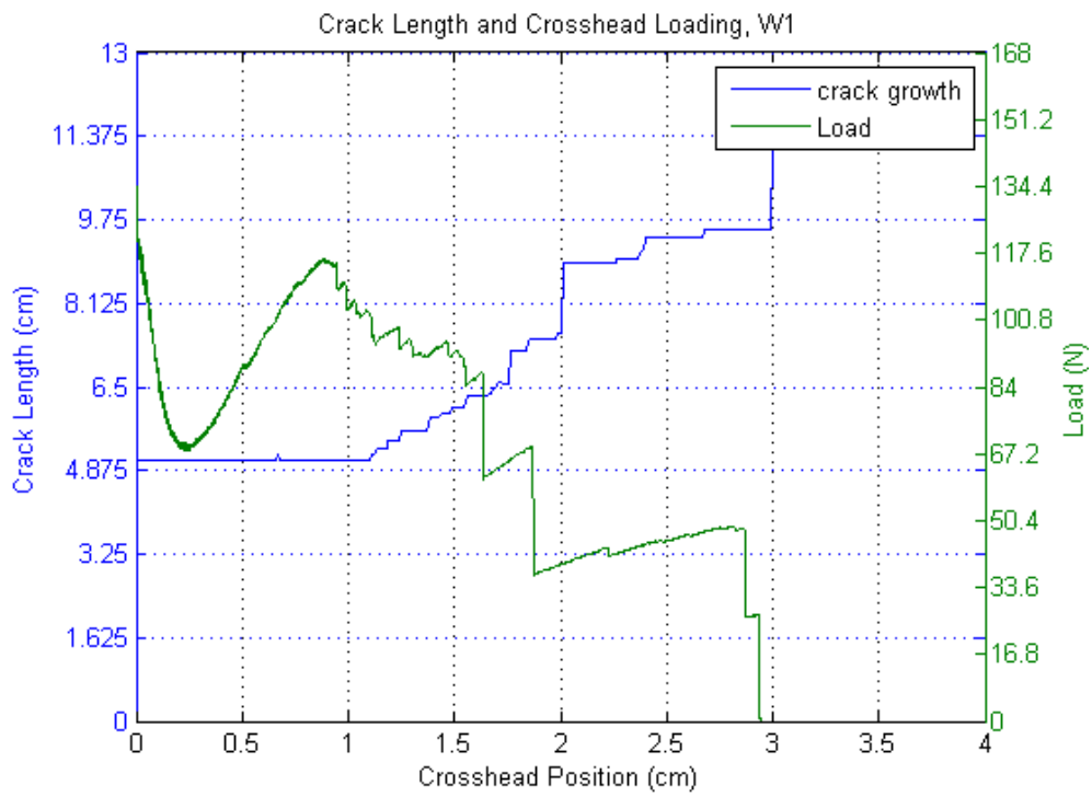
Figure 4.31: Crack length and crosshead load vs. crosshead displacement, Water Control.
