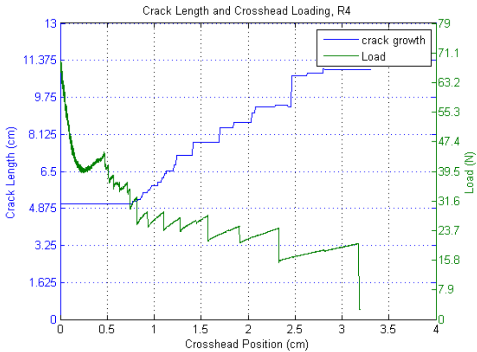
Figure 4.15: Crack length and crosshead load vs. crosshead displacement, 3-row injected CNF.
