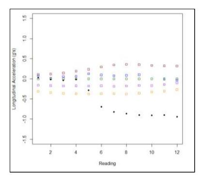
Figure 17. Crash comparison (black dots) with baseline readings.
