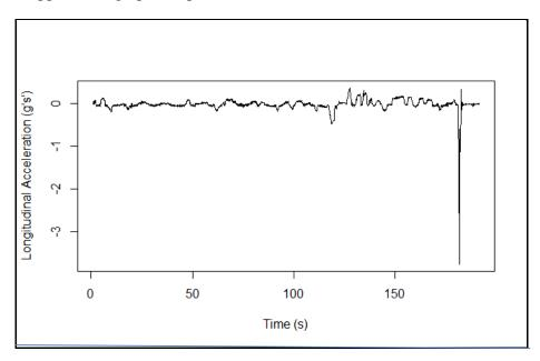
Figure 14. Sample time series of longitudinal accelerations, rear-end crash at time 170 seconds.
