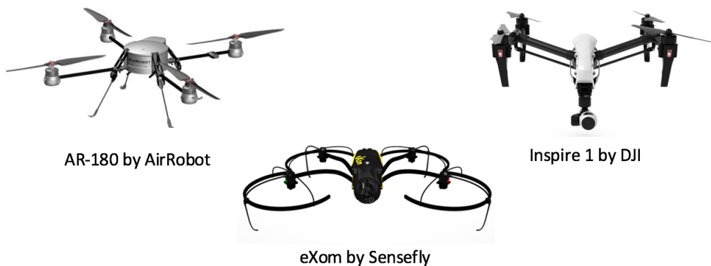
Figure 1.8: UAVs used for inspection; AR 180, Inspire 1, eXom [10] [13] [14]
