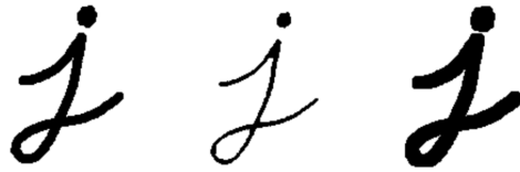
Figure 2.4: Morphological Erosion and Dilation [22]
