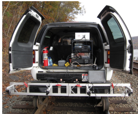
Figure 1.3: Camera setup of a hi-rail vehicle [8]
