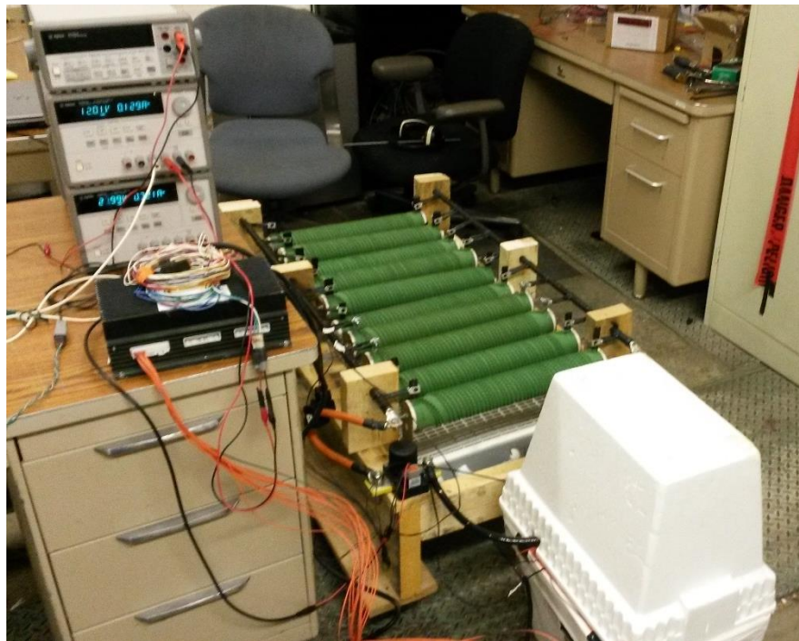
Figure 5.12 Full high amperage test setup. Styrofoam insulating box around batteries to help with temperature control.
