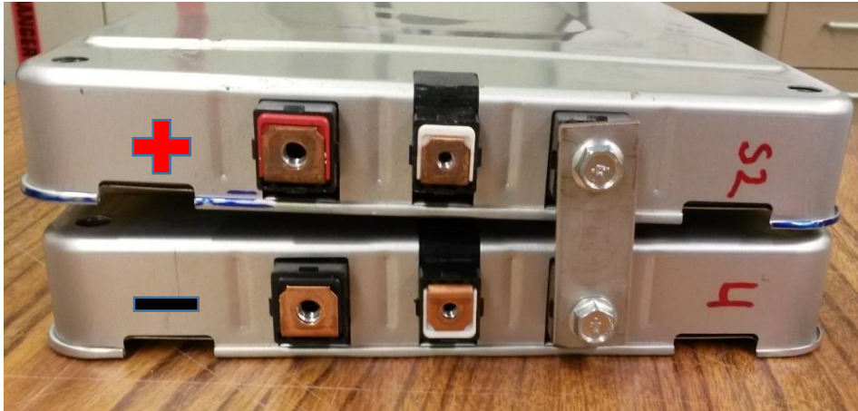
Figure 5.2 Battery configuration of physical batteries.
