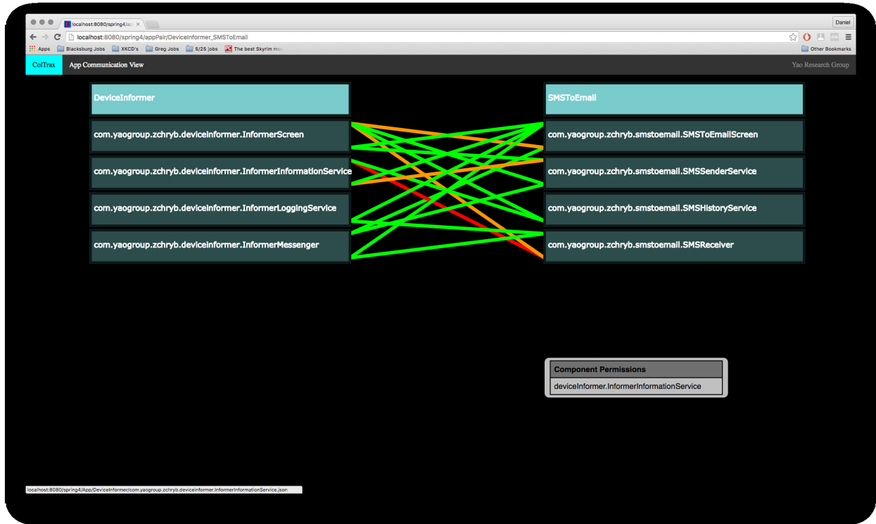
Figure 5.10: ICC view where a protected component is being hovered over.
