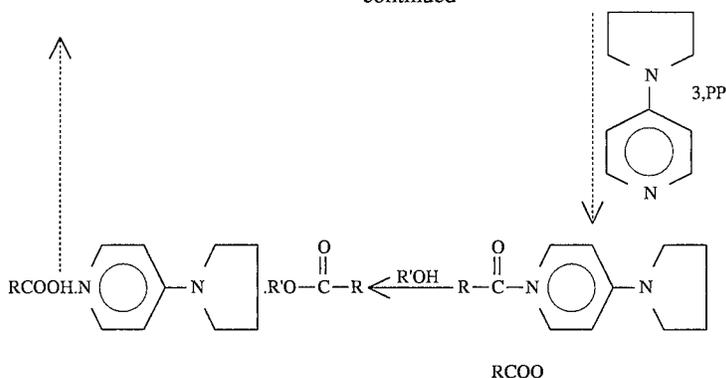
By recycling the spent half of the anhydride, its concentration in the medium is kept constant. 4-pyrrolidinopyridine (PP) converts the anhydride into a highly reactive species which reacts readily with an alcohol to yield an ester. The base is used only in catalytic amounts (e.g., 0.01 eq/OH).
