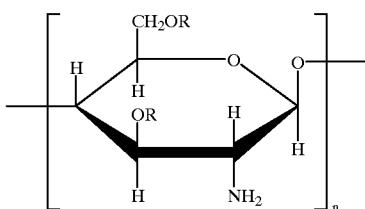
where n is greater than 3, and R is hydrogen or a one to twelve carbon (C<sub>1-12</sub>) ether or ester.
