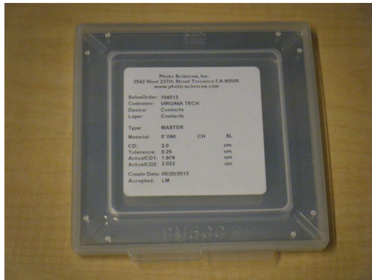
Figure (5.5): The photolithography mask used to make the testing pads for the nanostructures. It is a soda lime 4" chromium on glass mask with the smallest dimension on the mask being 0.5 \mu\text{m} .
