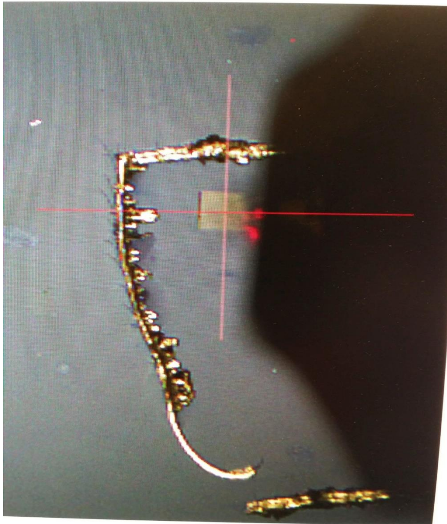
Figure (5.36): Nonspecific binding of gold particles to the entire surface remains a problem for constructing nanowires using nanografting. After we dipped the samples in colloidal gold nanoparticle solution we noticed that the gold nanoparticles have deposited on the entire sample. As the AFM tip scans the surface while we are imaging the patterns we constructed we noticed that it is shaving some of the weakly adsorbed gold nanoparticles from the surface. This can be seen in the above image as a lighter color square right underneath the tip marking the area which was scanned by the AFM.
