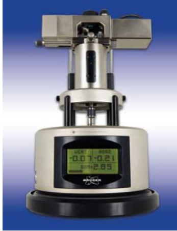
Figure (3.9): The MultiMode AFM system. It is capable of performing contact, non-contact, and tapping mode imaging. It utilizes a Veeco IV controller. This system is known for the high resolution it offers. (20) Reproduced with permission from: www.bruker.com
