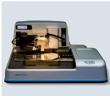
Figure (3.10): Dimension Icon ® is an AFM system that offers great nanoscale manipulation tools. It is equipped with a closed-loop scanner offering great precision for repositioning the tip on the sample. It has a piezo scanner based on a piezotube. (20) Reproduced with permission from: www.bruker.com
