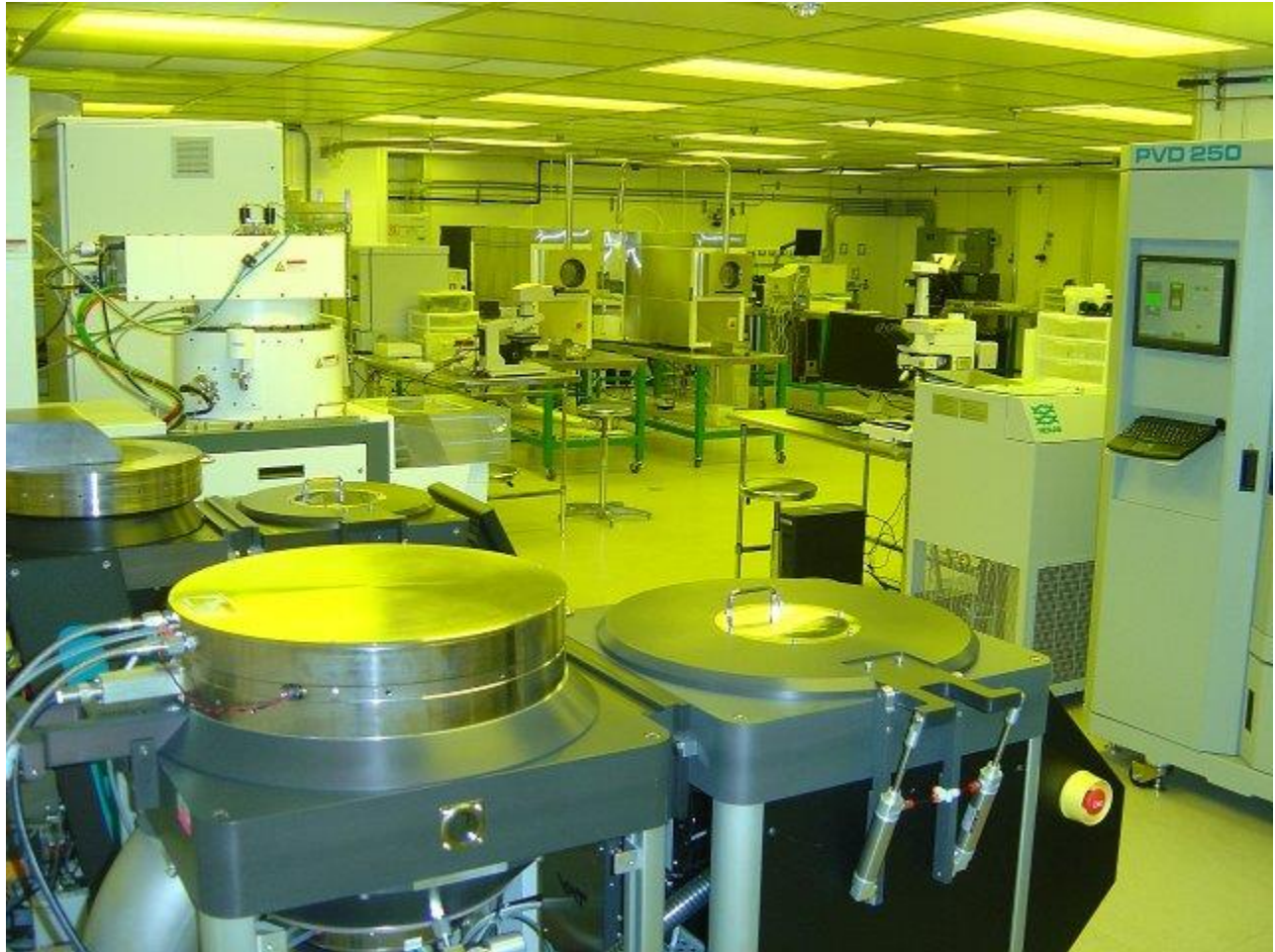
Figure (5.6): The cleanroom facility at Virginia Tech is a 1900 sq foot class 100 facility equipped with all equipment needed for a wide range of semiconductor micro-fabrication processes.
