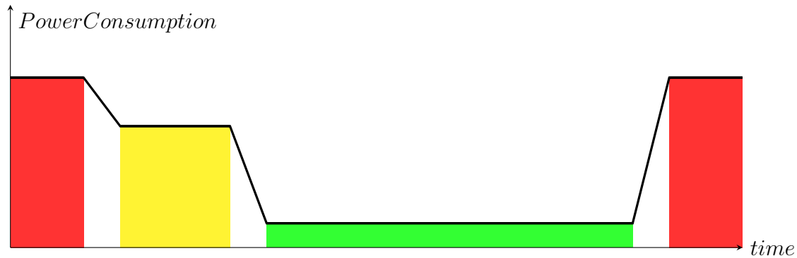
Figure 2.3: A timeline of a functional unit in a traditional power gating scheme. There are 3 periods of note: active (red), idle (yellow), and asleep (green).
