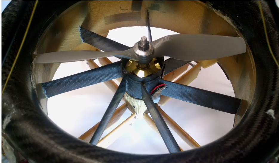
Figure 3.2: Image of the static veins and the propeller inside the duct of the vehicle
