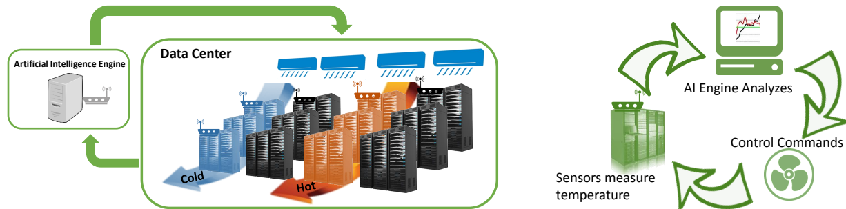
Figure 1.1: An example of a data-driven closed loop temperature control system of a data center.
