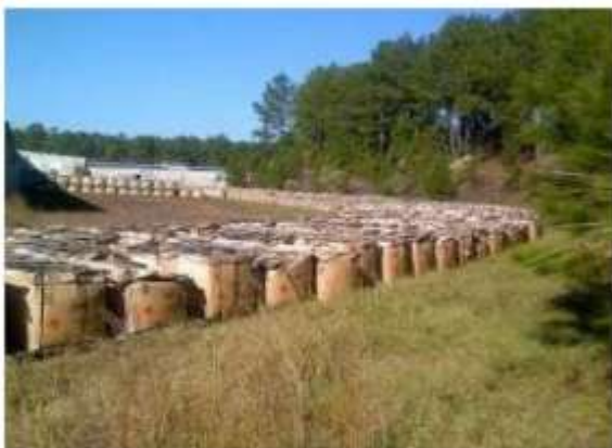
Photo 1: M6 Propellant improperly stored outside by Explo
