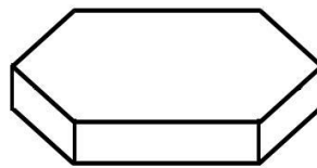
FIGURE 5.4(a) Hexagonal Disk-shaped Aggregate
