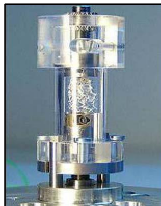
FIGURE 5.11 Testing Stage of the Microscopy System
