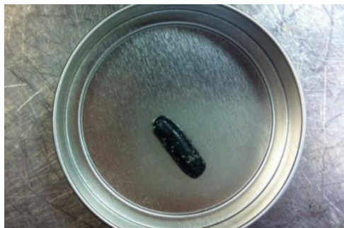
FIGURE 5.13 Asphalt Mixture Specimen Used in Compression Test
