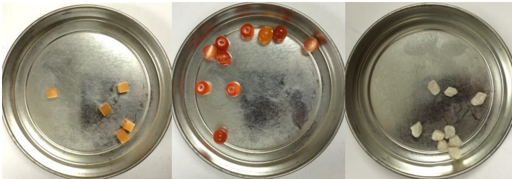
FIGURE 5.12 Crystal Particles and Aggregates Used in Compression Test
