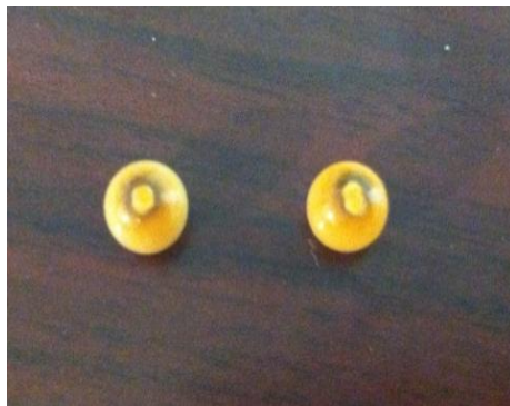
FIGURE 4.5 Crystal Aggregates Used in Compression Tests
