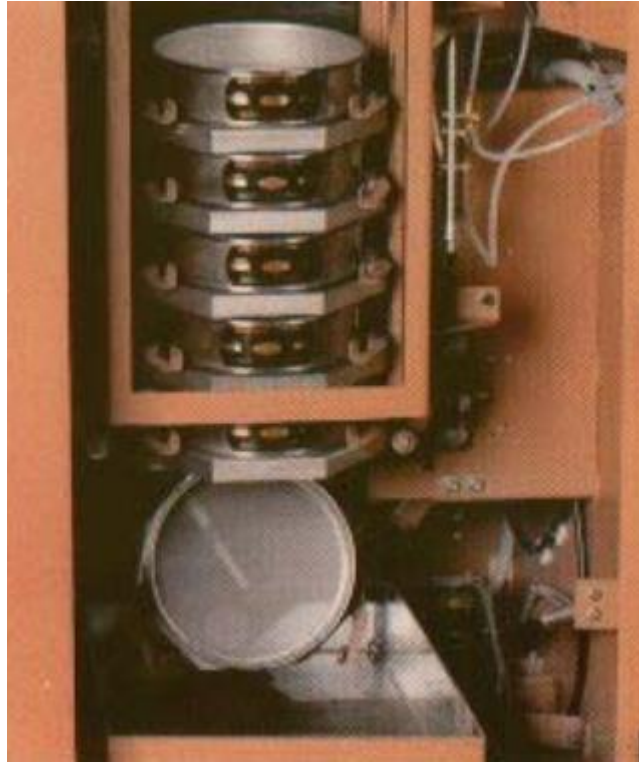
FIGURE 2.2 Gradex 2000 Sieve Configuration (9)
