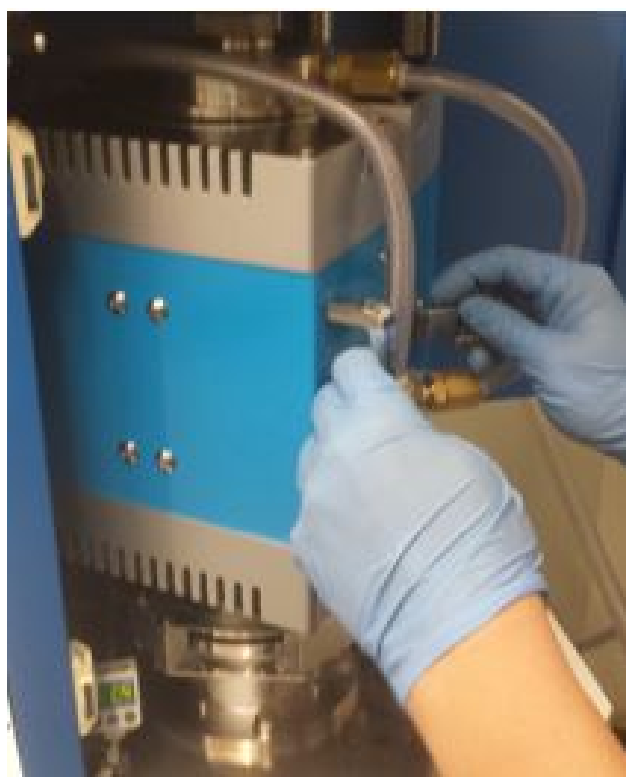
Figure 5.6: This is the photo of the heater for the laser flash rig.
