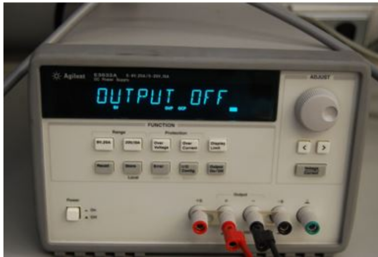
Figure 4.2: This is the Agilent E3633A ammeter, which was used to supply 10 Amps to the test specimen.
