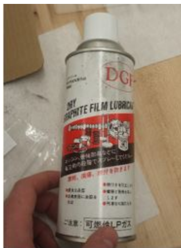
Figure 5.2: This is a photo of the graphite spray used on the sapphire and copper test pieces.
