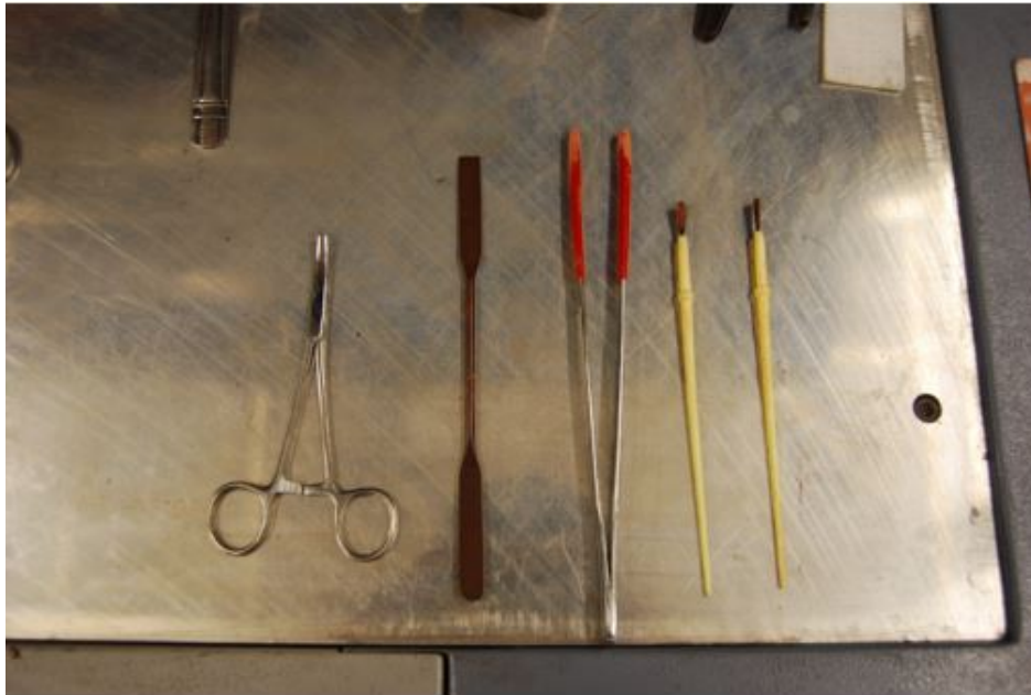
Figure 3.5: The instruments used to manipulate the test specimens to the ceramic kiln trays.
