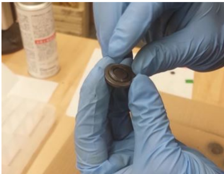
Figure 5.4: Placing the binder jetted copper pieces into the testing rig.
