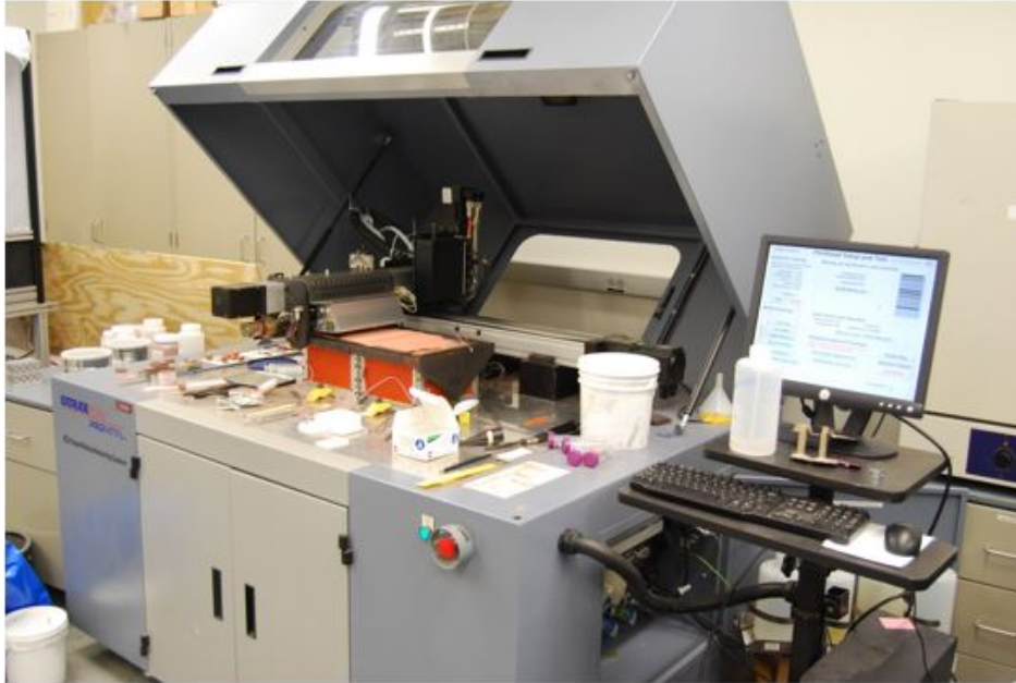
Figure 3.2: The Binder jet printer used to print the test samples.
