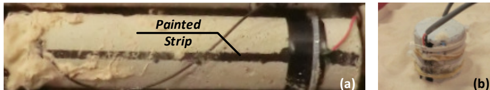
Figure 3.1. First Approach: Using Conductive Carbon Painting on a Soil-Cement Column, (a) Column with Painted Strip after Test, (b) Details of the Top of the Column in Soil Model
