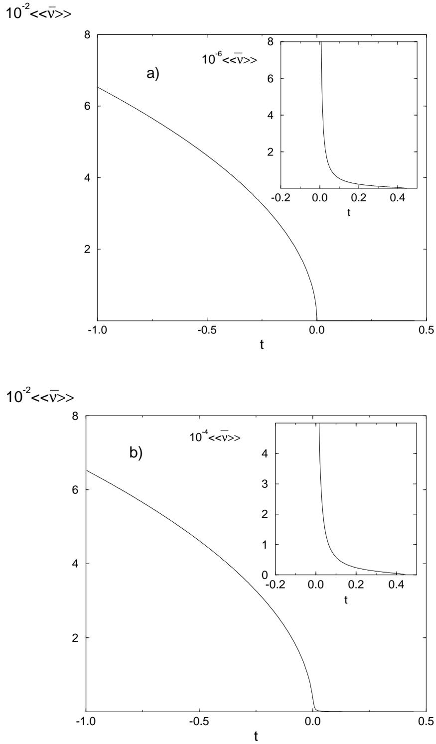
FIG. 2. Average order parameter  $\langle\langle\bar{v}\rangle\rangle$  vs. reduced temperature  $t$  for  $n_D = 10^{-5}$ ,  $\lambda = 3.0994 \cdot 10^{-11}$ erg (a), and  $n_D = 10^{-3}$ ,  $\lambda = 3.0949 \cdot 10^{-11}$ erg (b). The temperature range near  $t_c(n_D) = 0.444$  is displayed in the insets. Note the different scales of the two insets; the disorder strength was adjusted to yield the same  $T_c(n_D)$  in both cases (a) and (b).
