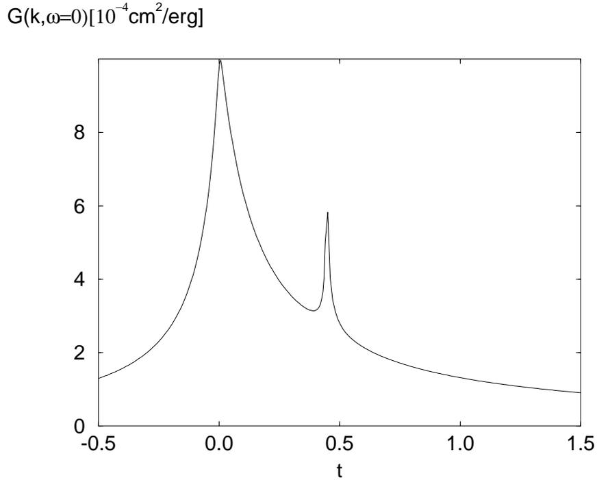
FIG. 5. Static phonon susceptibility (inverse elastic constant)  $G(\mathbf{k})$  [in  $10^{-4} \text{cm}^2 \text{erg}^{-1}$ ] vs. temperature at fixed angle  $\theta = 0$ .  $t_c(n_D) = 0.444$ ,  $\zeta = ka_0/2^{3/2}\pi = 0.07$ .
