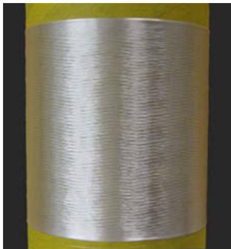
Figure 2-14. 560 m of hybrid dry-jet, gel spun VHMW PAN-co-MA fiber in 100 filament count tow ( 5.7 \pm 0.4 \mu\text{m} filament diameter, 1037 \pm 101 \text{ MPa} tensile strength, and 17.9 \pm 1 \text{ GPa} elastic modulus)
