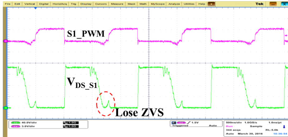
(a) Conventional ZVS detection method
