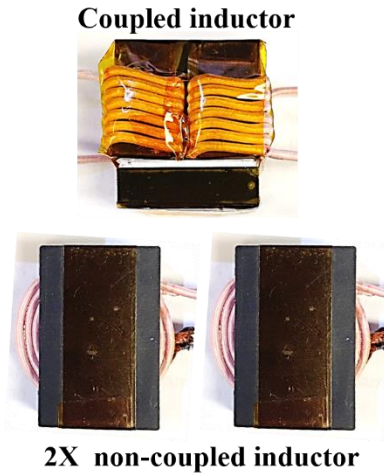
Figure B. 14 Comparison of coupled and non-coupled inductor
