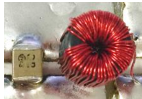
Figure 4.64 One-stage filter for proposed 150W 2-stage adapter
