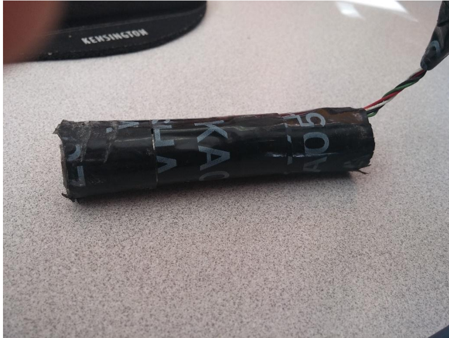
Figure 3.9: Force Transducer in Protective Plastic Jacket
