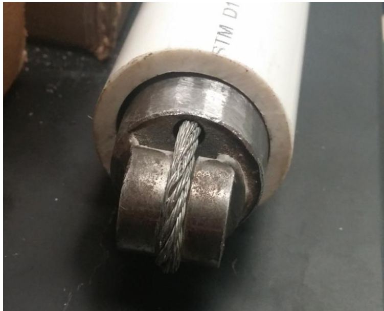
Figure 4.7: Scratch Head Embedded in PVC Pipe Walls Prior to Extraction
