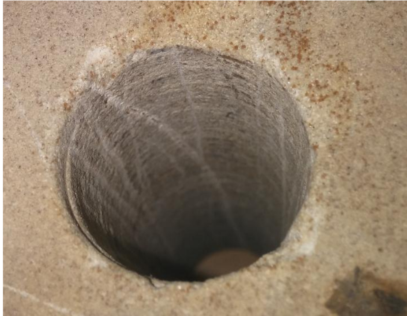
Figure 3.5: Scratch Demonstration on Sandstone Sample
