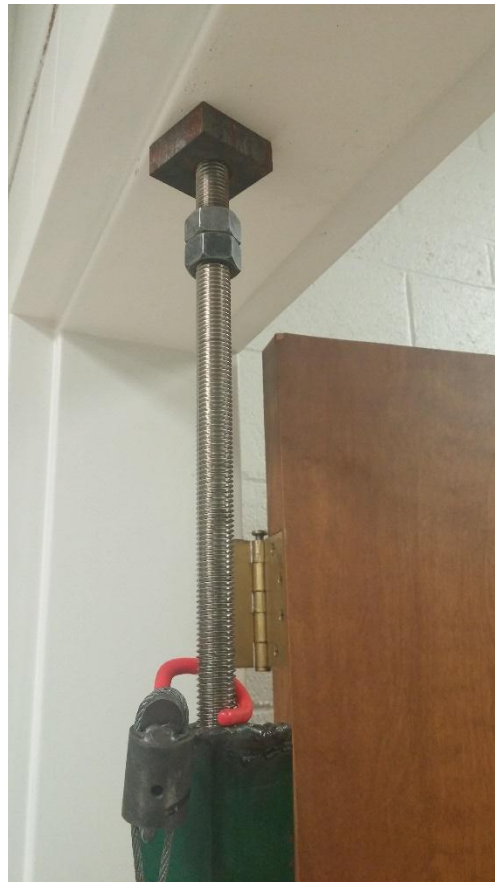
Figure 3.12: MRSAD Stand Screw Top and Brace Plate
