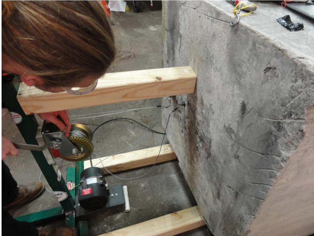
Figure 3.13: MRSAD Device with Wooden Braces for Horizontal Borehole Scratching
