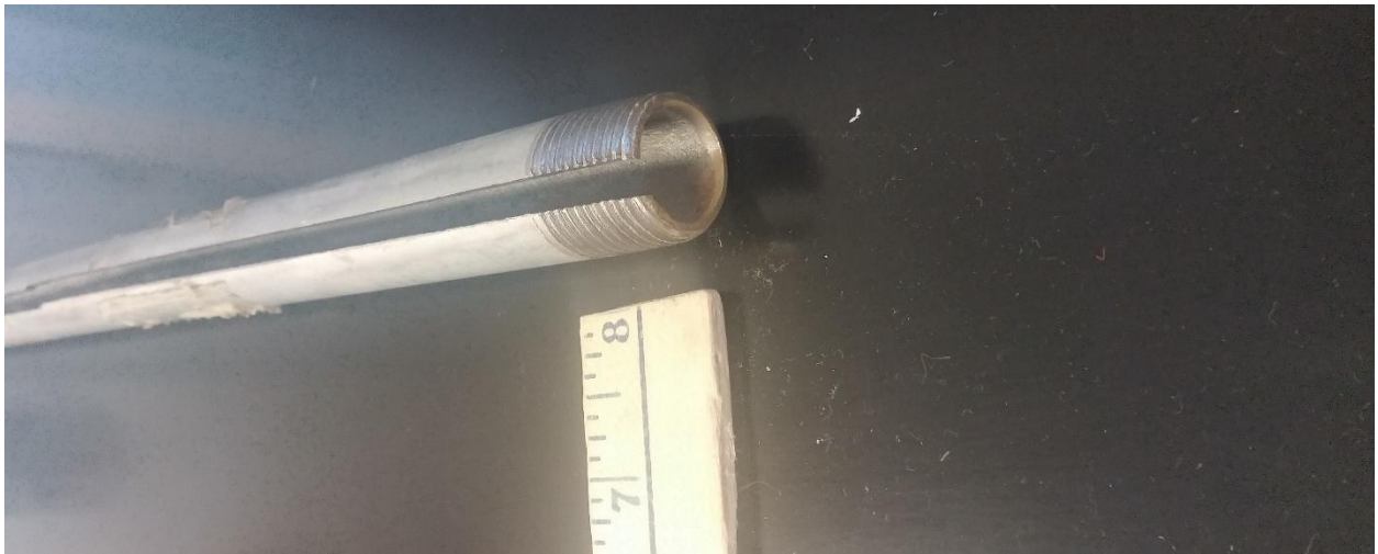
Figure A.8: Close View of Installation Rod Showing Cutaway Along Length for Removal Around Wiring
