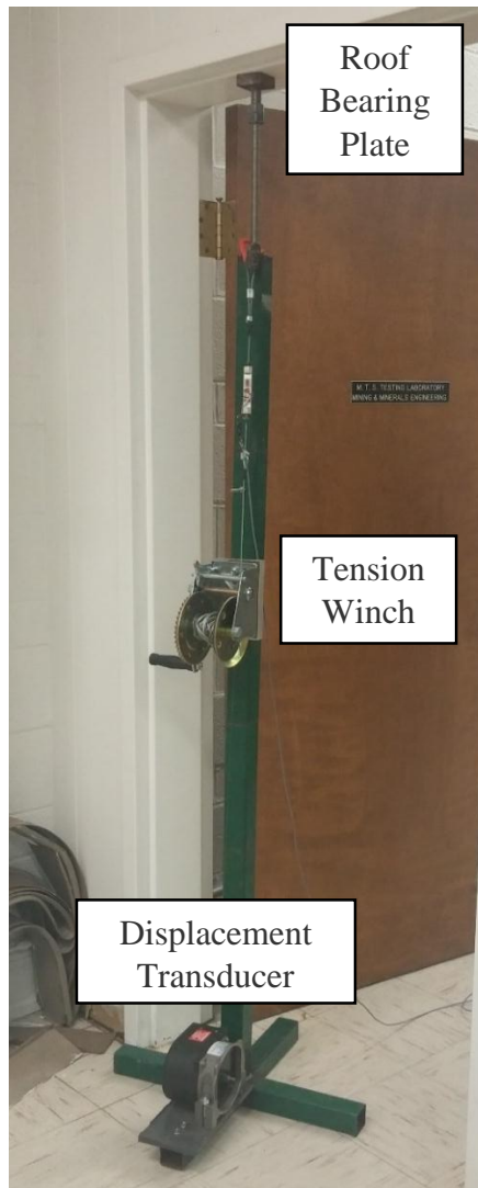
Figure 3.11: MRSAD Mounting Stand with Tension Winch, Roof Bearing Plate, and Displacement Transducer
