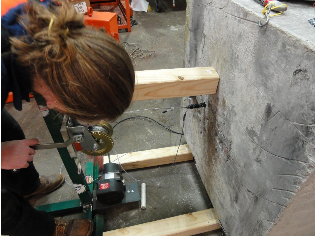
Figure A.4: Force Transducer Pulling from Concrete Block, Displacement Transducer Visible at Base of Green Stand
