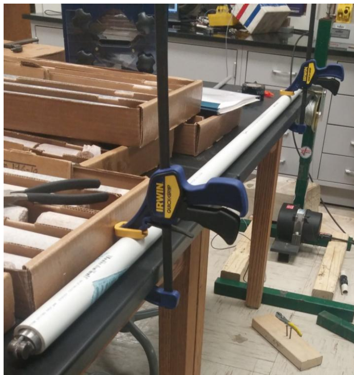
Figure 4.6: Clamped PVC Pipe with Scratch Head Visible Emerging from Pipe
