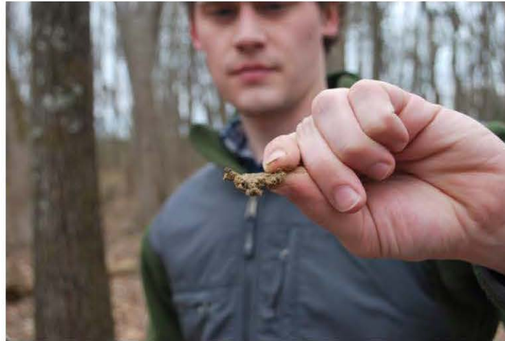
Designer Harley Walker performing a soil ribbon test on-site to quickly get an understanding of the soil's clay content.
