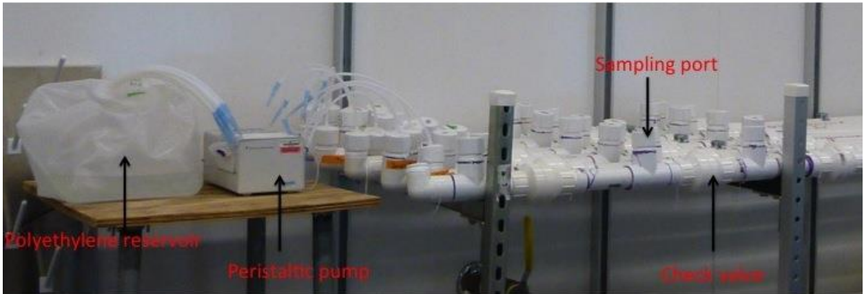
Figure A1: Photograph illustrating design of simulated distribution system (SDS).
