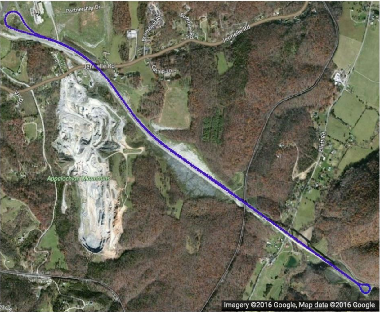
Figure 16. Smart Road course for dynamic platoon test.
