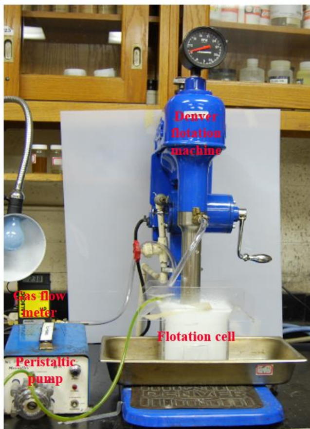
Figure 4.4 Equipment used to measure the bubble sizes in the froth.
