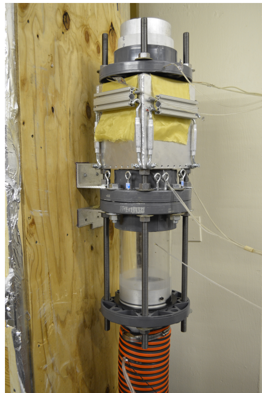
Figure 4.7: Construction of the in-house porosity testing apparatus.
