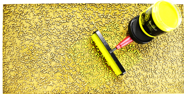
Figure 3.12: Tools used for speckling the Kevlar sheet: linoleum screen printing block, screen printing ink, and soft rubber brayer.
