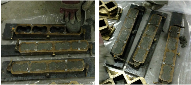
Figure 8.1: Mortar briquette specimens preparation.
