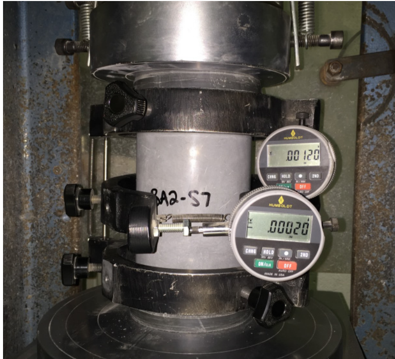
Figure 6.4: Poisson's ratio test setup.
