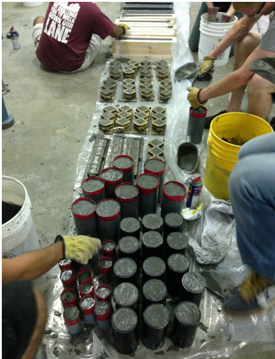
Figure 5.4: Batch-IV UHPC placement
