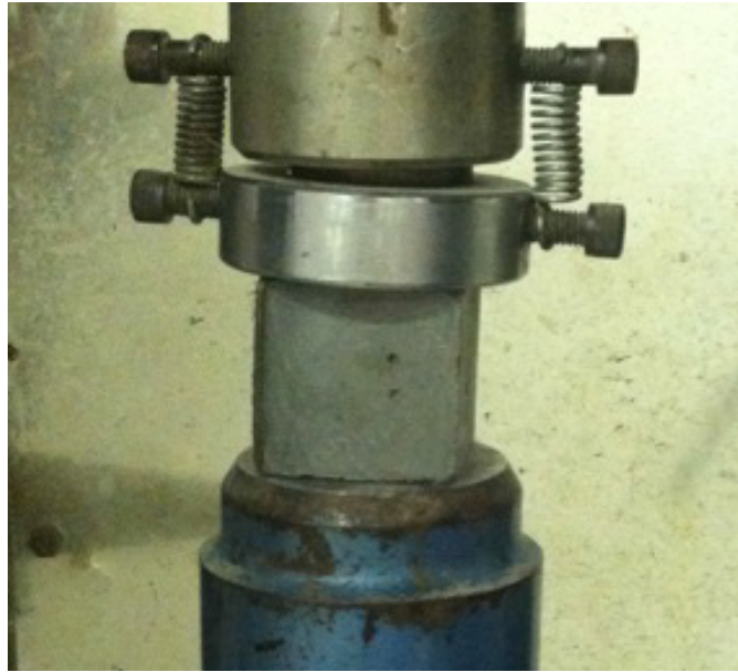
Figure 6.5: Cube compression strength test setup.
