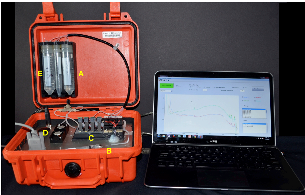
Figure 2. Seattle Sensor Systems Portable SPR Unit. The unit has a tube for buffer (A), a syringe for injection of a sample (B), 4 sensors (C), a peristaltic pump (D), and a waste container (E). The buffer (A) is pulled by a peristaltic pump (D) across the sensor surfaces and into a waste container (E). A syringe (B) is used to inject samples into an injection loop before the sample enters the flow cell. The flow cell is where the sample interacts with the sensor surfaces. Results are viewed on a laptop computer in real-time.
