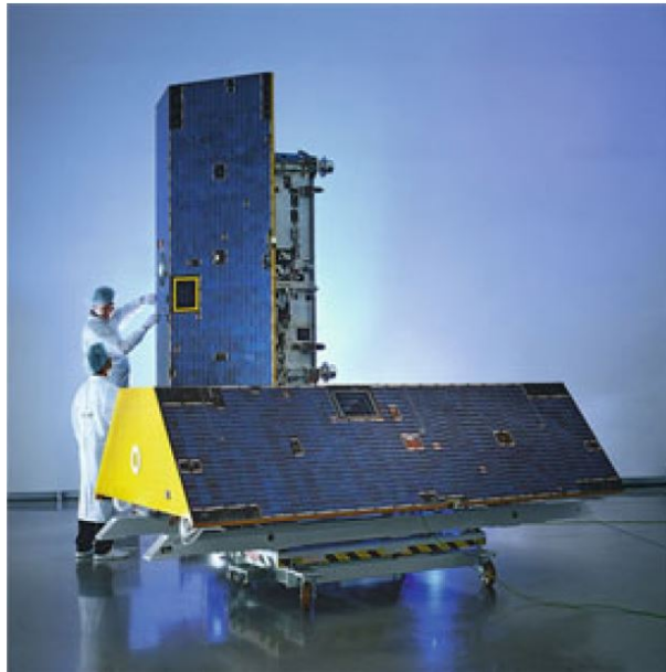
Figure 4.1: A photo of the GRACE satellites during integration from Doornbos (2012).
