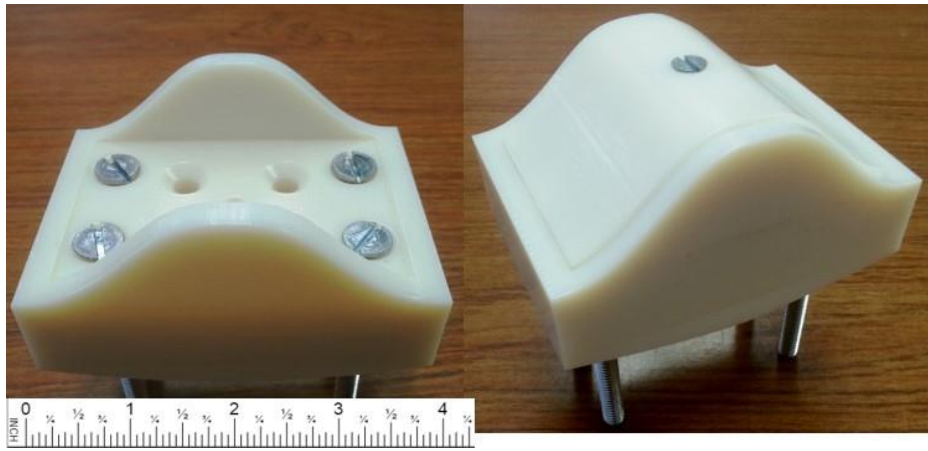
Figure 3.5: ICE 101 1/27^{\text{th}} scale strut balance mount.
