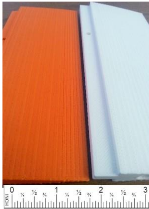
Figure 5.4: Flaps printed in horizontal orientation with visible stair-step surface finish.
