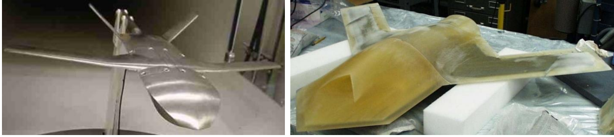
Figure 2.4: AFRL Striker Tanker SLS model at AFIT low-speed wind tunnel (left) and UCAV X45-A SL at AFRL Subsonic Aerodynamic Research Laboratory (SARL) (right). Tyler, C., Braisted, W., and Higgins, J. "Evaluation of Rapid Prototyping Technologies for Use in Wind Tunnel Model Fabrication," presented at the 43rd AIAA Aerospace Sciences Meeting and Exhibit, Reno, NV. January 10-13, 2005. AIAA-2005-1301. Used under fair use, 2015.
