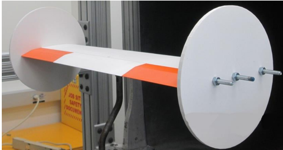
Figure 3.9: NACA 0012 airfoil with 8" endplates mounted in VT Open-Jet WT.
