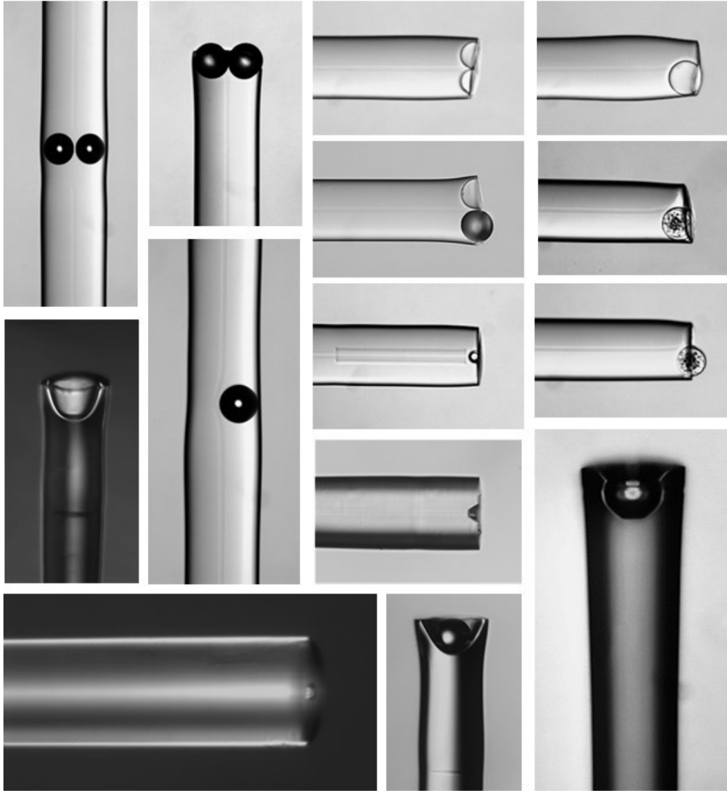
Figure B.0.1: Other candidate designs for in-fiber WGM resonators.
