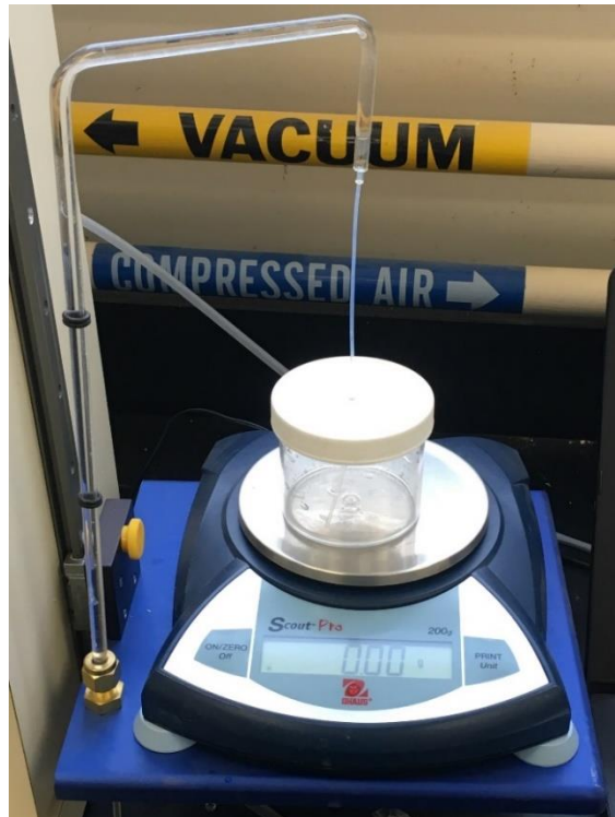
Figure 4.4. Effluent container and electronic balance
