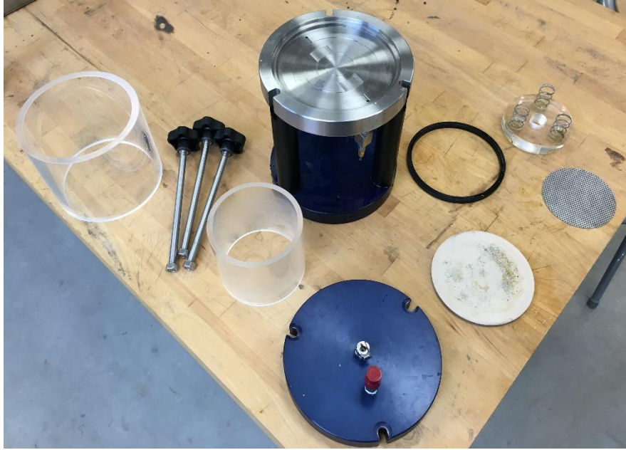
Figure 4.3. Main components of flow cell
