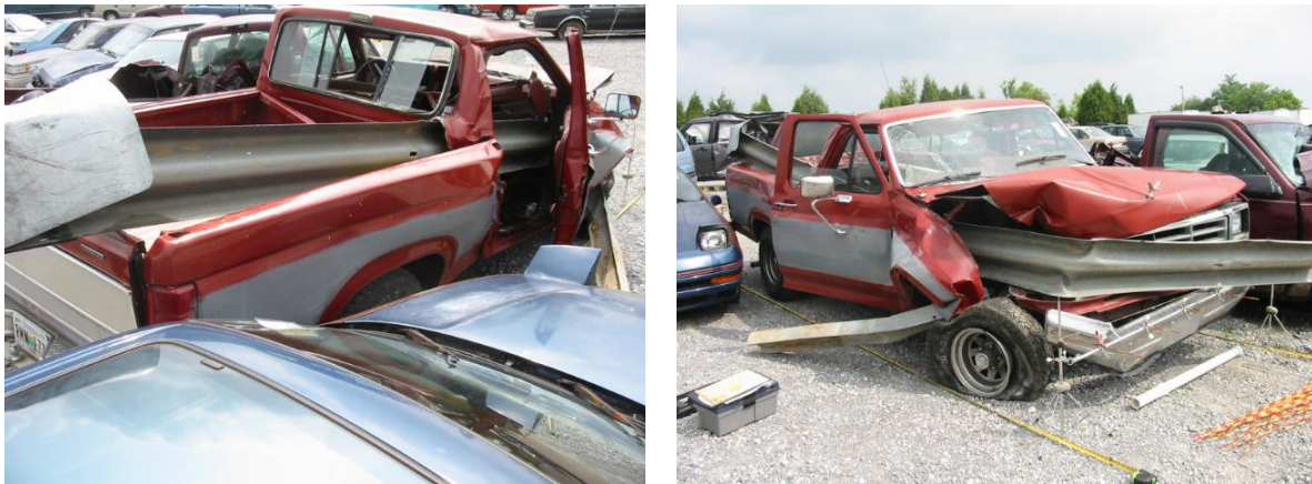
Figure A.1. The first guardrail end terminals were prone to penetrating vehicles that struck end-on. Newer end terminal designs aim to prevent this and bring striking vehicles to a stop without injuring vehicle occupants. NASS-CDS case 2005-45-104.
