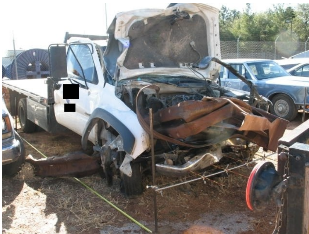
Figure 1.7. A guardrail end terminal embedded in the front of a crashed vehicle.
