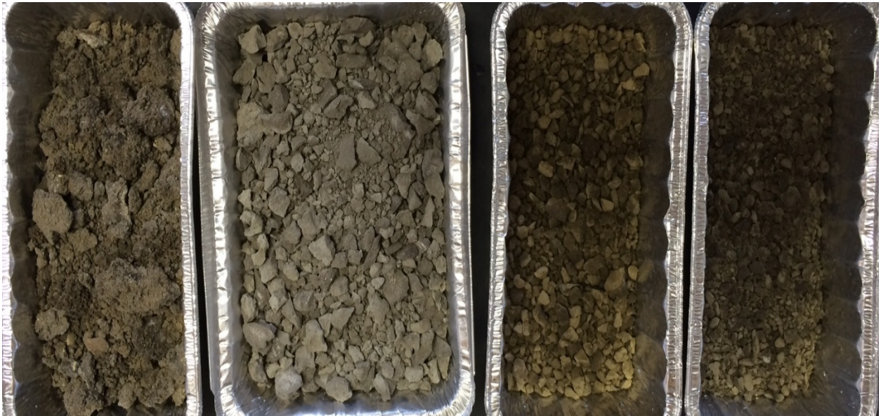
Figure 4-1: Dried, pre-ground samples in the following order: raw solids, solidified solids, drilling mud and treated solids
