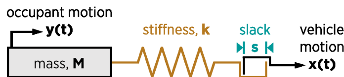
Figure 5.1 Schematic of the impact severity metric, vehicle pulse index (VPI), as a mass-spring system.
