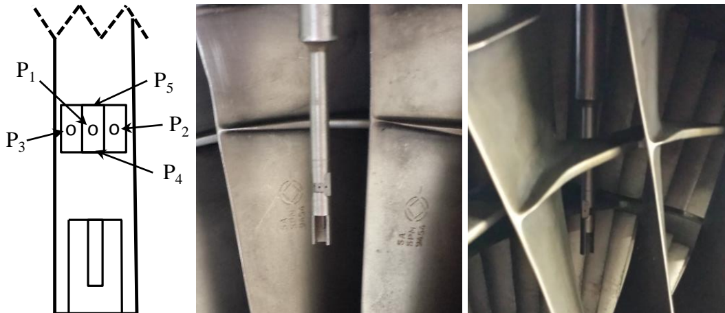
Figure 2.8. Five-hole probe schematic (left), fan inlet (Station 4) installation (center), and fan outlet (Station 5) installation (right).
