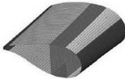
Figure.5.17. Mesh of the airfoil model in NASTRAN
