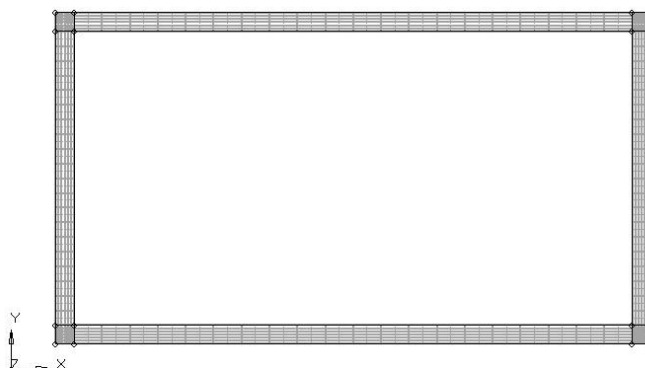
Figure.5.2. Rectangular box beam cross-section of the geometry.
