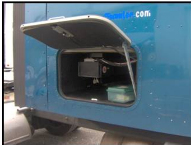
Figure 2. Photo. Encased computer and external hard drive installed in the truck's rear storage compartment.
