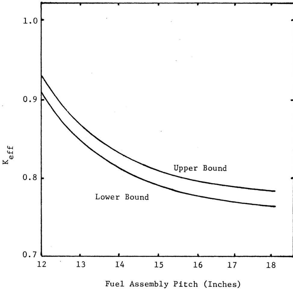
Figure 3.2. Typical Evaluation of  $K_{eff}$  for a New Fuel Storage Arrangement.
