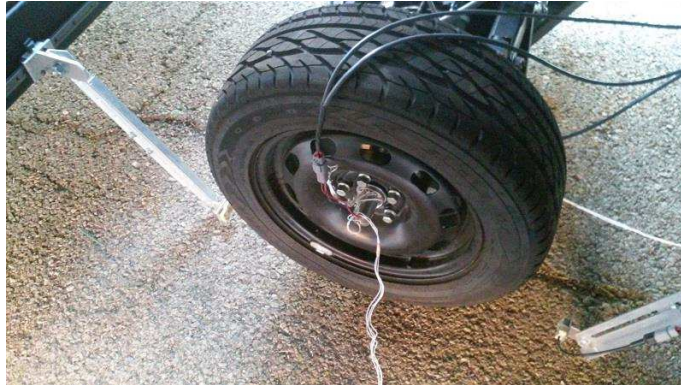
Figure 8.16: IR sensors at the entry and exit of the contact patch of the tire
