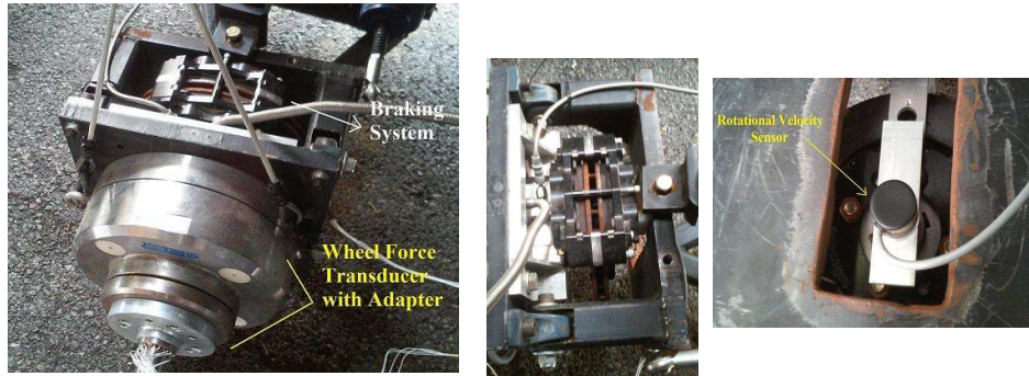
Figure 8.14: Wheel force transducer with braking system and rotational speed sensor mounted on to the shaft
