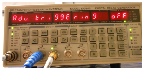
Figure B-5: Stanford Research Systems Model DG645 Digital Delay Generator is used to coordinate trigger to the Radar Digital Receiver and Digital Oscilloscope
