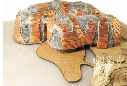
FACADE METAL SHEET SYSTEMS AND THE ETFE GLASS PANELS ARE APPLIED TO APPROPRIATE LOCATION
