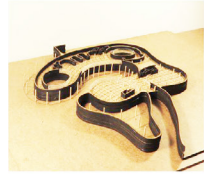
SECOND UNDERGROUND LEVEL IS BUILT AT 9 FT UNDER WATER LEVEL WITH THE RETAINING WALL AND STRUCTURE GLASS WALL TO ALLOW VIEWS INTO WATER
