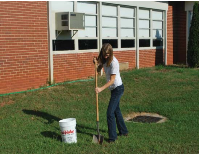
CDAC team member Tish Poteet conducts a percolation test of the courtyard soil.
