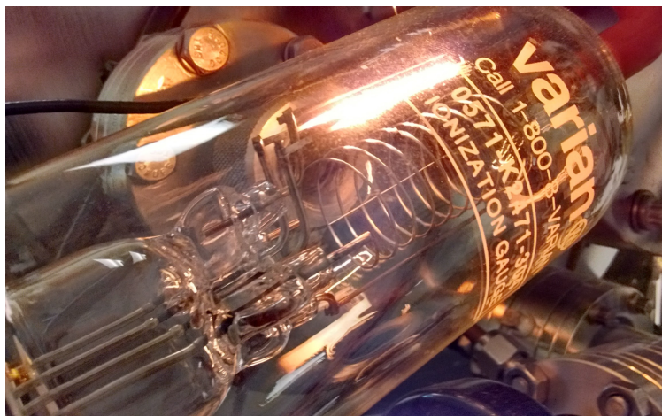
Figure 2.1: Close-up of a Bayard-Alpert type ionization gauge tube connected to the Space@VT vacuum chamber. Note the glowing hot filament electron source.
