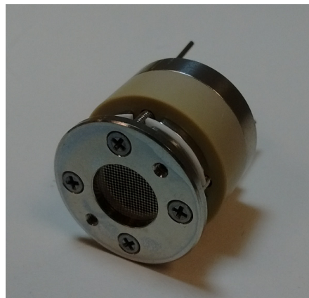
Figure 2.4: A Photonis APD microchannel plate device as used in the SNeuPI ionization chamber.
