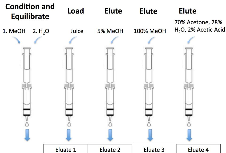
**Figure 6.3:** Diagram of the SPE method used to isolate polyphenol compounds from sugars in the juice matrix where Eluates 1 and 2 are expected to have the higher sugar concentrations and Eluates 3 and 4 are expected to have the higher polyphenol concentrations, based on the SPE cartridge chemistry as designed for sample prep methods.
