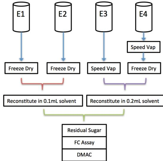
**Figure 6.4:** Diagram representing the sample preparation and analysis steps after SPE.
