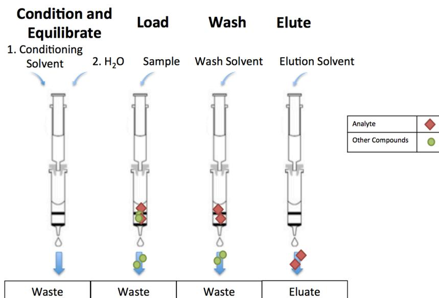
**Figure 6.2:** General procedure for SPE with a conditioning and equilibration step followed by loading, washing, and eluting.
