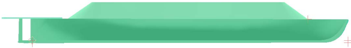
Figure 22: Ship's Reference Points. The Perpendiculars are referenced from the upper hash marks, and the Marks are referenced from the lower hash marks
