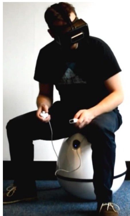
Figure2.11 – VRGO hands free movement device (Ryan 2015).
