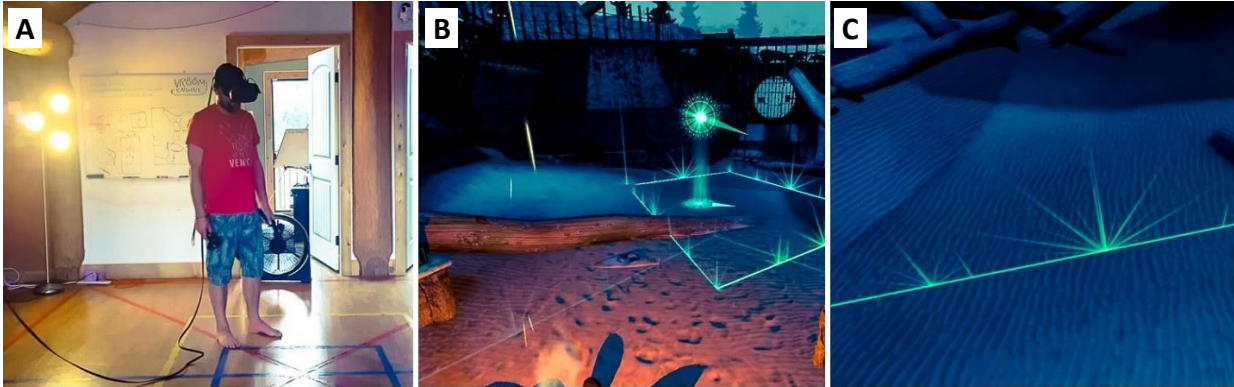
Figure 2.17 – Blink locomotion technique based on teleportation, A: The user can explore part of the VE as large as the physical space at each time, B: The user can move a representative of the physical space to explore other places in the VE, C: A visual effect shows the boundaries of the real world to the user
