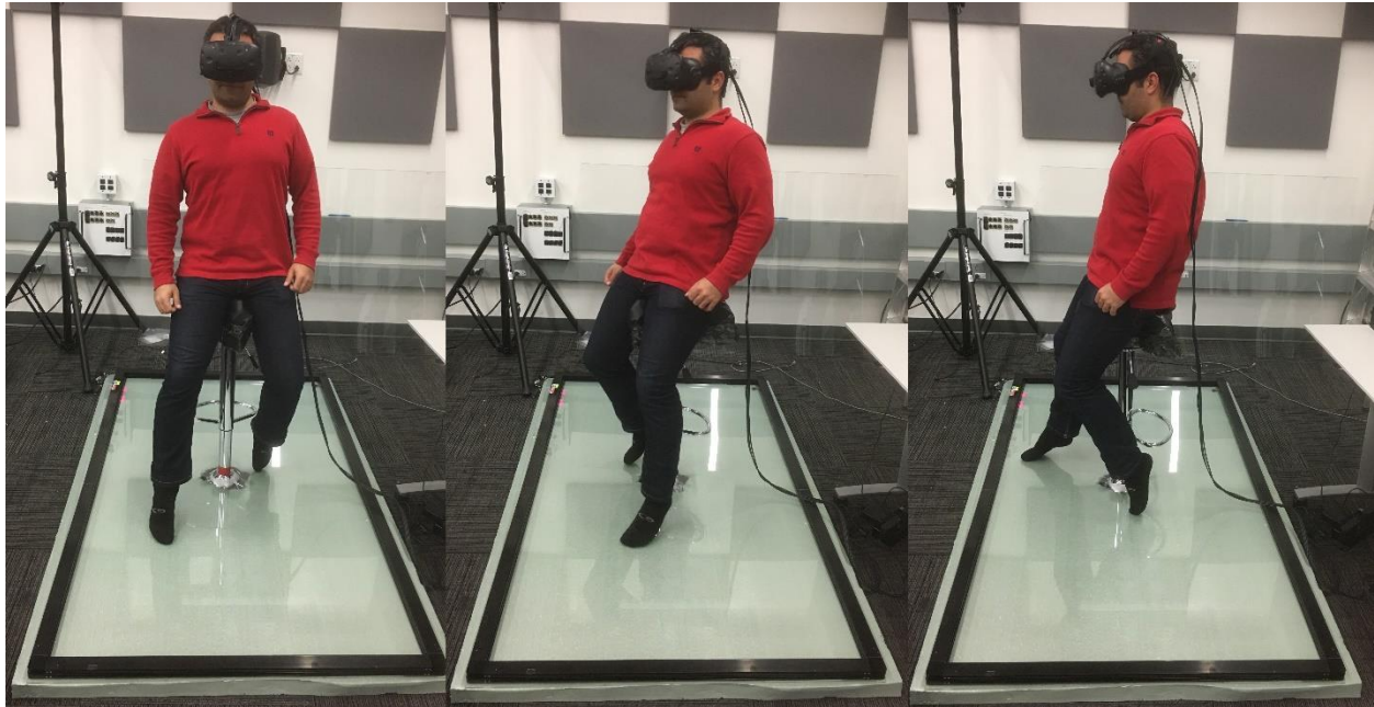
Figure 9.7: The final version of physical prototype of the novel locomotion interface working with an HMD display.
