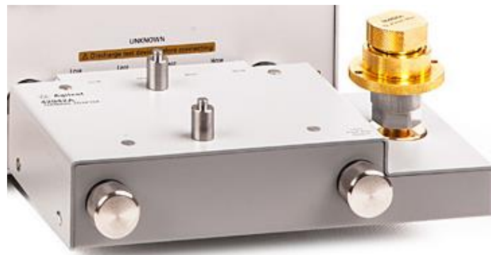
Fig. 16. Keysight 16454A fixture to test the complex permeability of the core [45].
